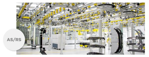
We designed a solution that combines automated storage (AS/RS) and transportation through overhead conveying systems. The ShopStocker is an overhead conveyor system with elevators between levels, which provides to your production chain a new way to transport and store a component of any nature.
