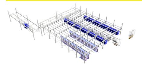
This system enables the management (storage and transportation) of work-in-progress parts.
