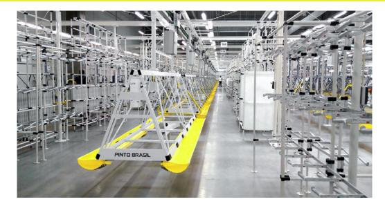
Optimized space utilization, overhead assembly lines are designed to make the most efficient use of available floor space. By moving assembly processes and materials overhead, they free up valuable floor real estate, allowing manufacturers to maximize their production capacity without the need for extensive facility expansions.
